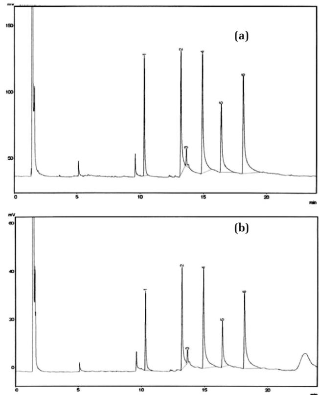
**Fig. 7:** The GC chromatogram representing (a) Standards in solvent, (b) Standards in matrix of Lettuce detected on FTD from methodology-II (1-Dimethoate, 2-Methyl parathion, 3-Chlorpyrifos, 4-Quinalphos, 5-Profenophos, 6-Triazophos).
