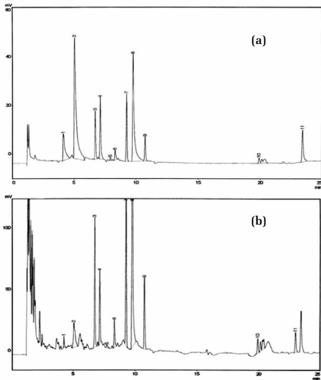
**Fig. 6:** The GC chromatogram representing (a) Standards in solvent, (b) Standards in matrix of Lettuce detected on ECD from methodology-II (1-Atrazine, 2-Chlorthalonil, 3- Methyl parathion, 4-Chlorpyrifos, 5-Captan, 6-Quinalphos, 7-Profenophos, 8-Endosulfan alpha, 9-Endosulfan beta, 10-Cypermethrin, 11-Deltamethrin).
