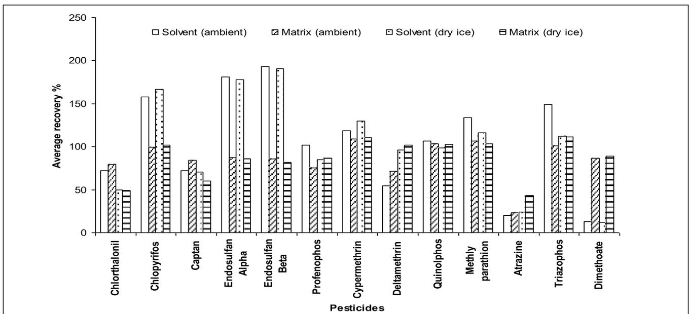
**Fig. 4:** Graph representing the average recovery of pesticides from solvent and matrix match calibrations of the Methodology II ambient and low temperature samples.
