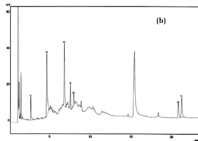
**Fig. 5:** The GC chromatogram representing (a) Standards in solvent, (b) Standards in matrix of Lettuce detected on ECD from methodology-I (1-Heptenophos, 2-Chlorthalonil, 3-Chlorpyrifos, 4-Captan, 5-Isofenphos, 6 & 7-Fenvalerate).
