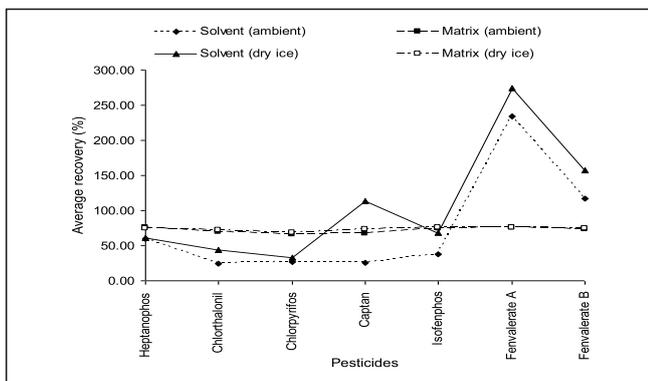
**Fig 3:** Graph representing the average recovery of pesticides from solvent and matrix match calibrations of the Methodology I ambient and low temperature samples.
